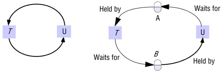
**Figure 16.21** A cycle in a wait-for graph
