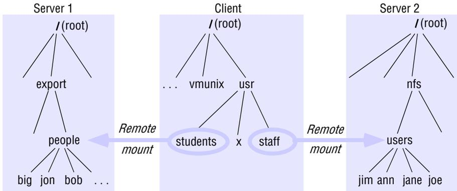
Note: The file system mounted at `/usr/students` in the client is actually the subtree located at `/export/people` in Server 1; the filesystem mounted at `/usr/staff` in the client is actually the subtree located at `/nfs/users` in Server 2.
