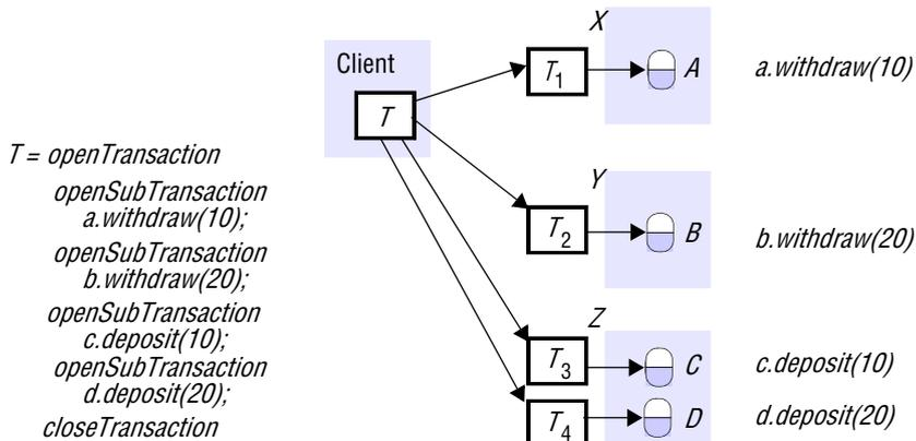
**Figure 17.3** A distributed banking transaction
