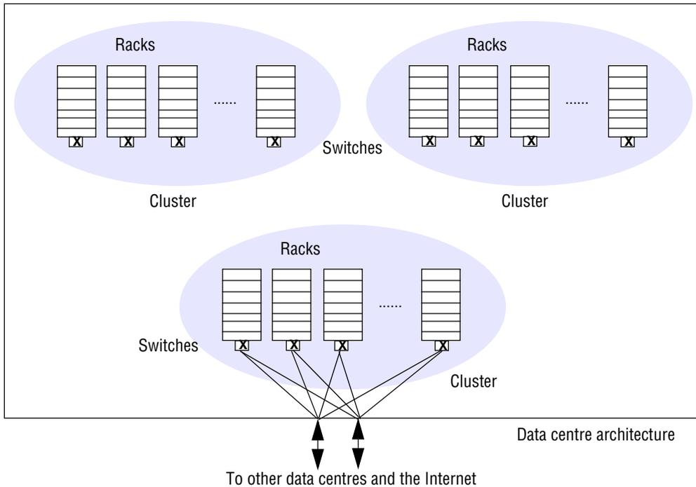
(To avoid clutter the Ethernet connections are shown from only one of the clusters to the external links)
