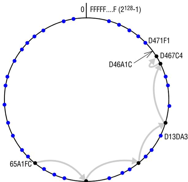
The dots depict live nodes. The space is considered as circular: node 0 is adjacent to node  $(2^{128}-1)$ . The diagram illustrates the routing of a message from node 65A1FC to D46A1C using leaf set information alone, assuming leaf sets of size 8 ( $\neq 4$ ). This is a degenerate type of routing that would scale very poorly; it is not used in practice.
